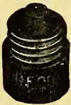
FIG. 311.—A plug fuse. Insurance rules have done away with the open string fuse originally used. This fuse screws into a lamp socket; the cover is of mica, for inspection.
